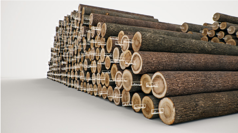
Every log stored in a pile has its "digital fingerprint" and is clearly identifiable.
